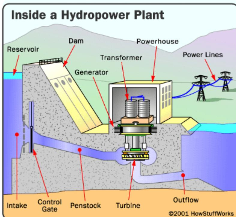
Figure 1: The design of a large hydro plant. Source: <http://people.howstuffworks.com/hydropower-plant1.htm>
